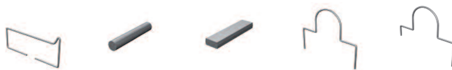
Driver worn out Stitching wire OK Stitching wire pressed flat Correctly preformed staple Leg too short
