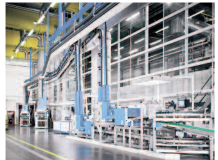
An overhead conveyor provides layout flexibility that is particularly important in narrow spaces and for linking up buildings or floors over long distances. Some systems can handle up to three shingle streams to transport a large number of copies per running meter at the lowest cost. Photo: Muller Martini Newsvevor
