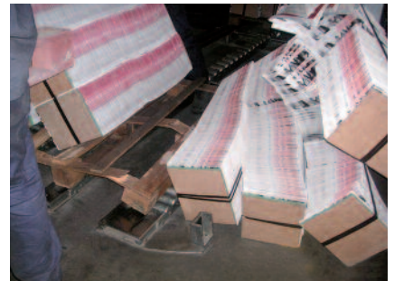
The consequence of using pallets in poor condition can be substantial damage to printed product and possible risk of accident. Photo: Muller Martini
