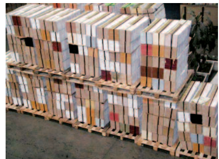
Incorrect pallet stacking can negatively impact signature quality, and can also be an accident risk. This photo shows the strap on logs in the lower pallet level are stretching which makes the second pallet from the right unstable.
