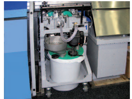
Cold glue station with integrated glue bucket.
