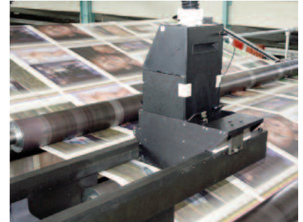
Inkjet imprinting systems integrate easily with web offset presses and web finishing equipment to allow printers to leverage their existing assets by adding value to direct marketing and other jobs and extend their business opportunities. Photo: Kodak
