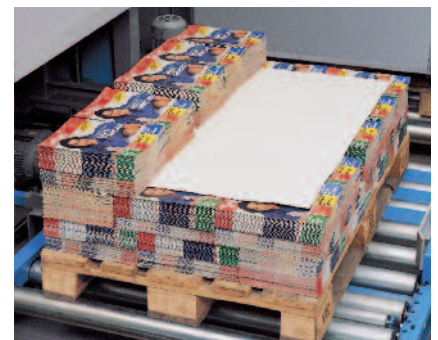
A slip sheet between the layers increases the stability of the pallet load. Photo: Muller Martini
