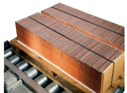
Correctly prepared logs are less subject to damage when palletised. Photo: Muller Martini
