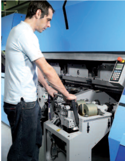
Interchangeable glue station in perfect binding line. Photo: Muller Martini
